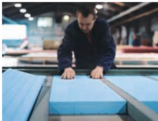
Fig. 13 >> Inserting the STYROFOAM™ boards into a floor panel.
