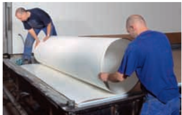
Fig. 09 >> Applying facing layer (GRP in this illustration)
