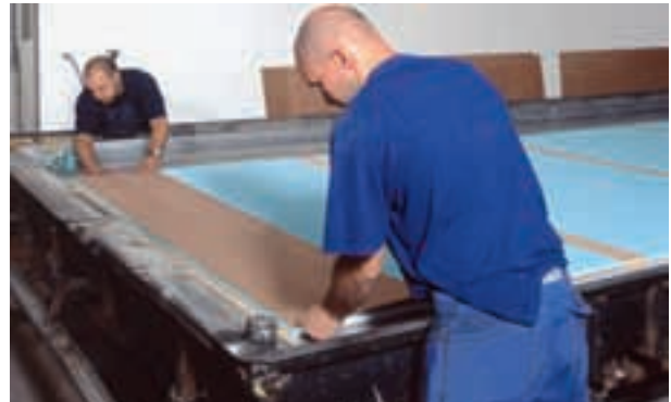
Fig. 08 >> Once the adhesive has been applied, a laminated wooden layer is installed
