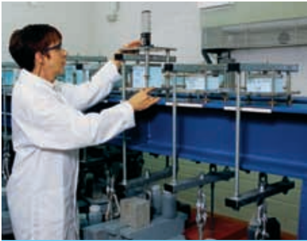
Fig. 10 » Creep testing STYROFOAM™ in the laboratory
