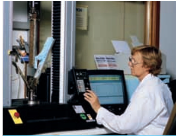
Fig. 11 » Shear test on STYROFOAM™
